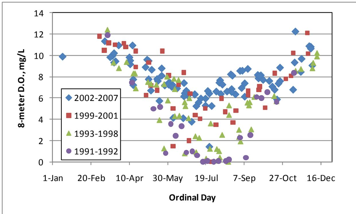
Figure 7. Deep water (8 meters below surface) dissolved oxygen concentrations in Bear Creek Reservoir, 1991-2007. The data are aggregated across years by plotting against ordinal day. Years are segregated according to aerator technology (see Table 1): 1991-1992 – no aeration; 1993-1998 – hypolimnetic aeration without disrupting stratification; 1999-2001 – full water column aeration with barrel aerators; 2002-2007 – full water column aeration with pan diffusers.
